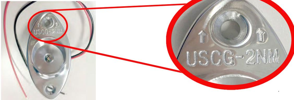
2. These lights are designed to be mounted on a vertical surface 24 degrees relative to the boat's centerline so that the light pattern is unobstructed. International Navigation Rules require that sidelights be installed above the uppermost continuous deck, i.e. above the vessel's rub rail.
